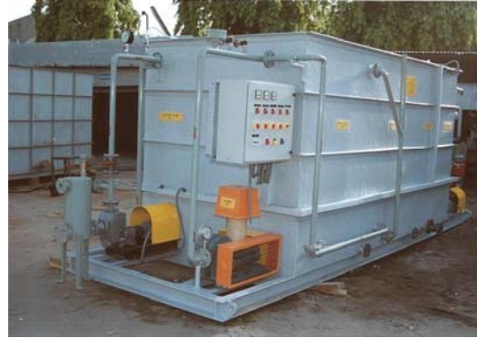
Domestic Sewage: Package Moving Bed Bio reactor plant at a resort in South Africa.
